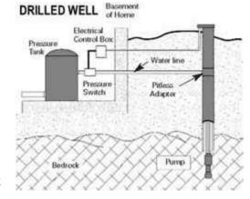
the well. By law, the casing has to extend at least 18 feet into the ground, with at least 5 feet extending into the bedrock. The casing should also extend a foot or two above the ground's surface. A sealant, such as cement grout or bentonite clay, should be poured
